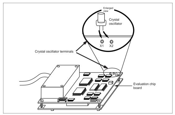
Figure 9 Installing the Clock Oscillator
